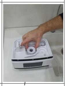
Water filter that needs replacing to prevent limescale deposits from being blown into the room. Important: Soak the water filter in tap water for 2 hours before inserting it into the humidifier. This helps to activate the filter for it to work at maximum efficiency.
